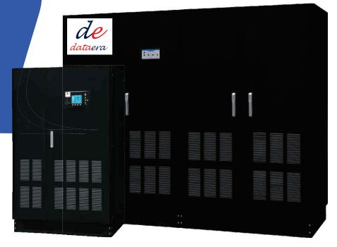
Dx890 series UPS 80  $\sim$  500 kVA provide maximum protection and power quality for mission critical loads, including data centers, Industrial Processes, telecommunications, security and electro-medical systems. It is on-line double conversion UPS with IGBT based 3-level PWM rectifier technology, featured with high input power factor (> 0.99), low THDi, high efficiency and built-in output isolation transformer.
